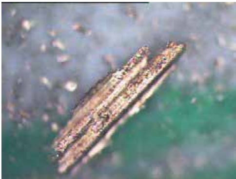
Figure 5 - 400 micron slip wear particle
