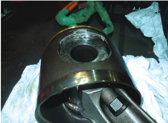
Figure 3: Silver wrist pin bearing was damaged.
