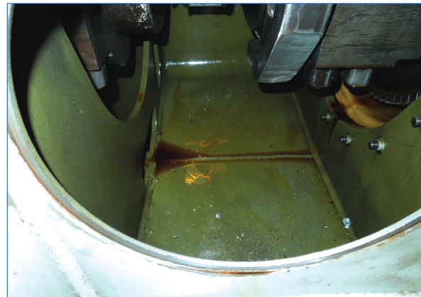
Figure 2: Silver-coated bearing material identified in the engine crankcase.
