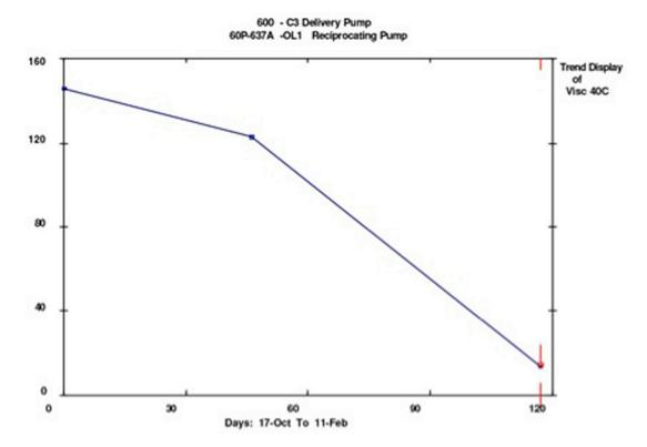
Viscosity is a lubricant's internal resistance to flow at a given temperature (40° C) in relation to time and is considered to be the single most important physical property of a lubricant. Changes in viscosity indicate improper servicing, dilution, contamination or lubricant breakdown in service. Viscosity is usually determined with a kinematics method and the results are reported in centistokes (cSt).
