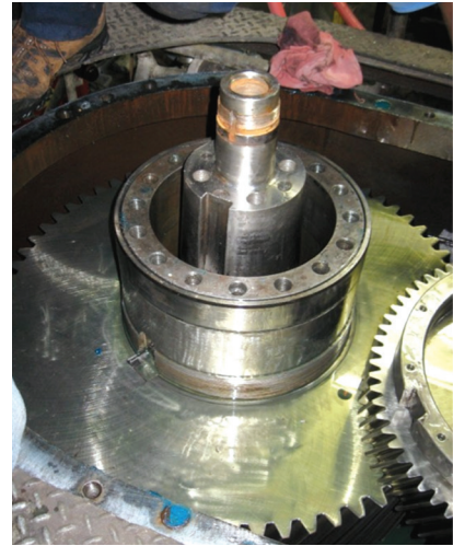
Figure 3 - Autoclave bearing and shaft cap removed revealing the underlying gearing. Cooling water is directed down the hollow center portion of the shaft
