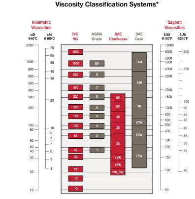
\*This grade comparison is a general guide that applies to viscosity at several different reference temperatures but does not evaluate total lubricant quality. These comparisons are based on a 95 VI product.
