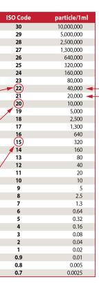
Particle count results are assigned three ISO code numbers based on the total number of particles equal to or greater than a given size range.
