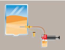
Samples drawn from a common return line collection point provide superior accuracy when the valve is installed upstream of the filter. This is the best sampling method for assessing machine contamination.
