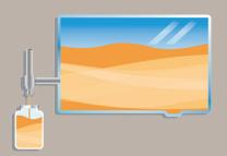
A permanent sampling port provides a consistently accurate sample collection source and is applicable to both pressurized and nonpressurized systems.
